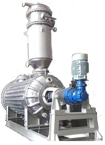
Rotary Vacuum Paddle Dryers (RVPD) is a cylindrical jacketed vessel with a central agitator having specially designed blades. The blades of this Rotary Vacuum Paddle Dryer (RVPD) are so designed that they sweep the entire internal surface and at the same time turn the material so that all the particles are come in contact with the heated surface.
